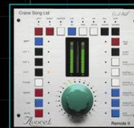
9. Crane Song Avocet Our discrete class A monitor controller, our sound brain that assures the perfect audition.
